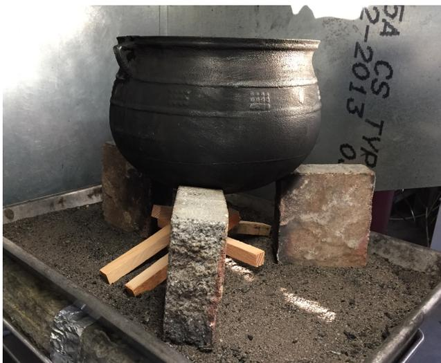
**Figure S1.** Three-stone fire arrangement with Darfur pot.
